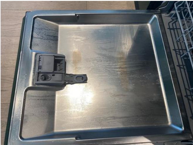
Discoloured marks to interior dishwasher door
